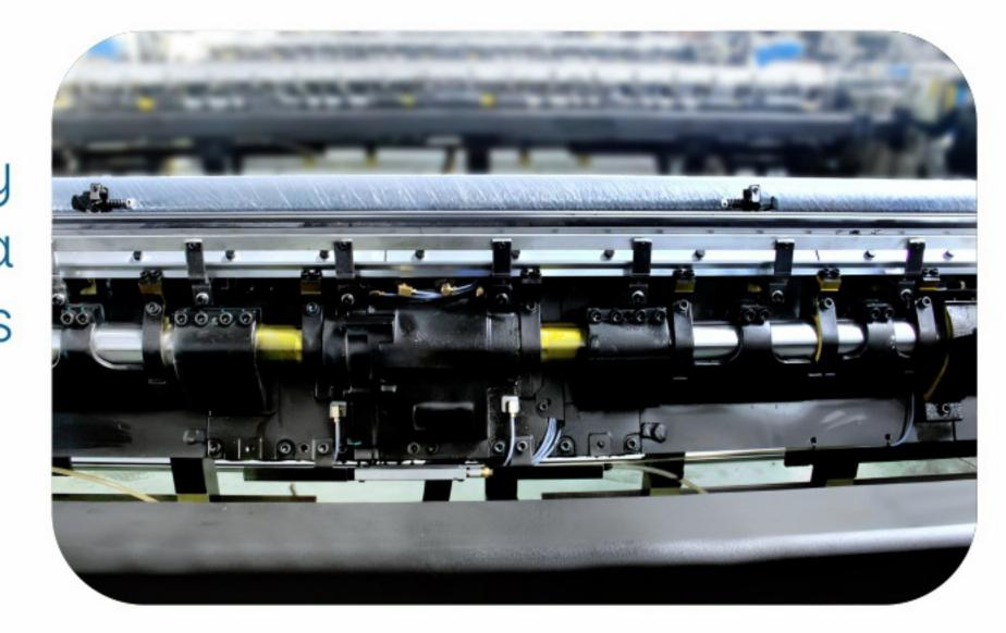
**Dolphin 999** offers unique full leno selvedge motions which are electronically driven by individual stepper motors. They are mounted in front of the harnesses, so that all harnesses remain available for fabric pattern formation.
